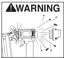
Exceeding the maximum permissible operating pressure may cause the nailer to explode, blowing metal fragments in all directions. To protect yourself from serious personal injury, DO NOT allow your air compressor to exceed the recommended pressure when connected to this nailer!
